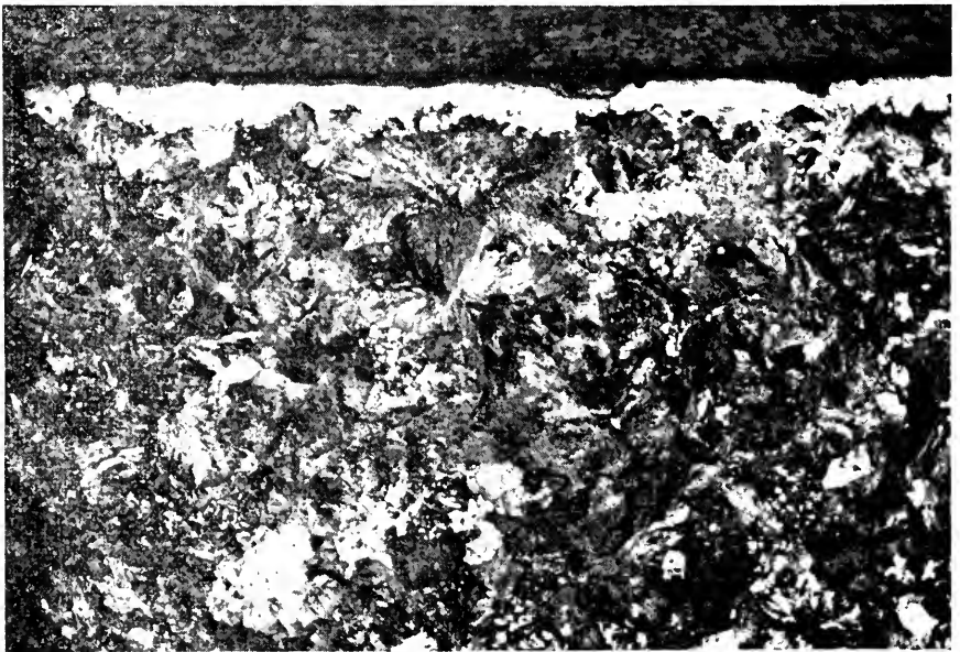
Fig. 18 (Investigation 136-31)—Photomicrograph of a specimen that was cut through the fatigue ring development shown in Fig. 17. It can be noted that a layer of martensite was round at the origin of this failure. This martensite formation is the result of a heavy grinding of the collar after the thermite weld metal had cooled.
